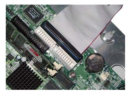
Every motherboard has at least two such ports. To install Open-E iSCSI, you have to use the first (primary) port.
